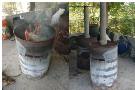
Fig. 5. Biochar steel furnace.
