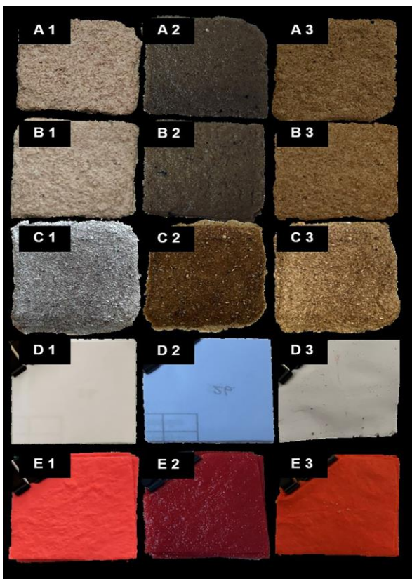
Fig. 6. Photographs of the fiber sheets prepared from waste lingzhi mushroom bed after pretreated with 9.5% w/w NaOH for 120 min (A), and 13.5% w/w NaOH (B); C) fiber sheet with 40wt% binder; D) printing paper and; E) mulberry paper. The number of 1-3 mean the sample before soaking in water, after soaking in water and after soaking in water and left at room temperature for 16 h, respectively.
