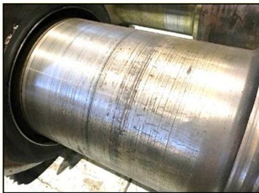
(b) Roller shaft failure
