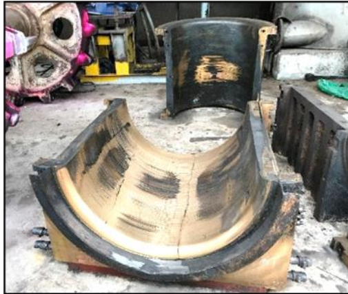
(a) Journal bearing failure
