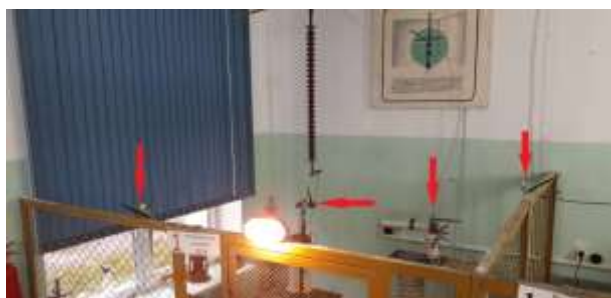
Fig. 9. Insulator LK 70/110 with sensors installed around in the laboratory.
