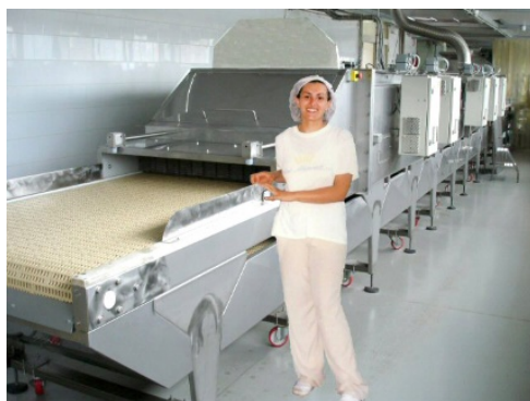
Fig. 2. System used for drying sweets and vegetable products [15]
