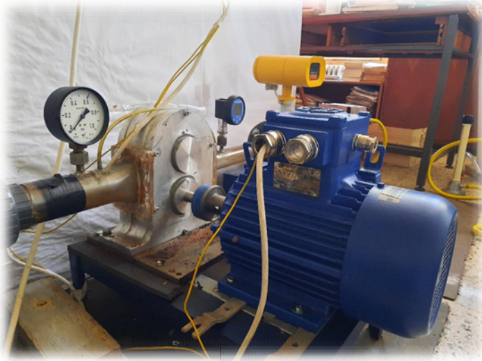
Fig. 5. Overview of the volumetric pump in the test stand.
