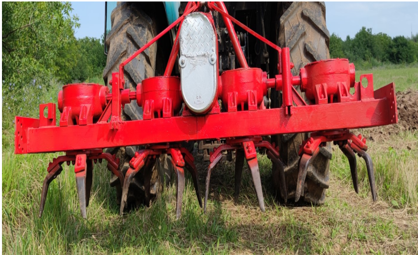
Fig. 1. Detail of the four rotors that equip the agricultural harrow with vertical rotors.
