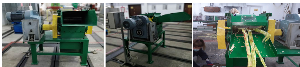
Fig. 1. Equipment for pressing sorghum stems to obtain bioethanol
