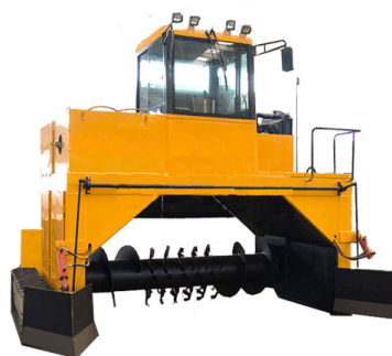
Fig. 3. Crawler Type Compost Turner equipment [18]
