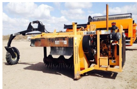
Fig. 5. WILDCAT compost turner equipment, model LS117A [20]
