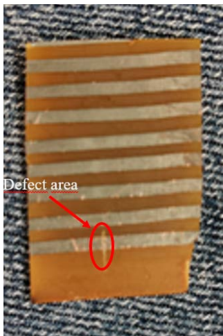
Fig. 8. Defective track located near other conductive tracks, track width is 1.5 mm, distance to an adjacent track is 0.9 mm, defect width is 0.1 mm
