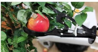
Fig. 14. Process of conducting a laboratory experiment, capturing the fetus with a developed device
