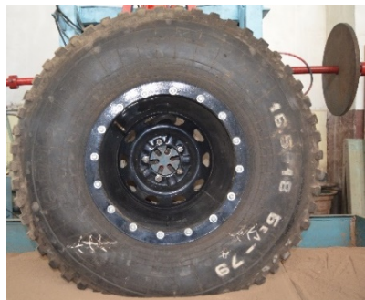
Fig. 9. Loss of shape of the sidewall of 1020x420-18 tire at an air pressure of 10 kPa and a load of 5.15 kN.
