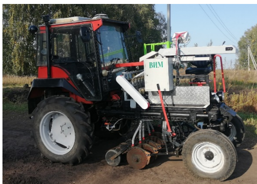
Fig. 1. Self-propelled seeder with multi-level seeding system
