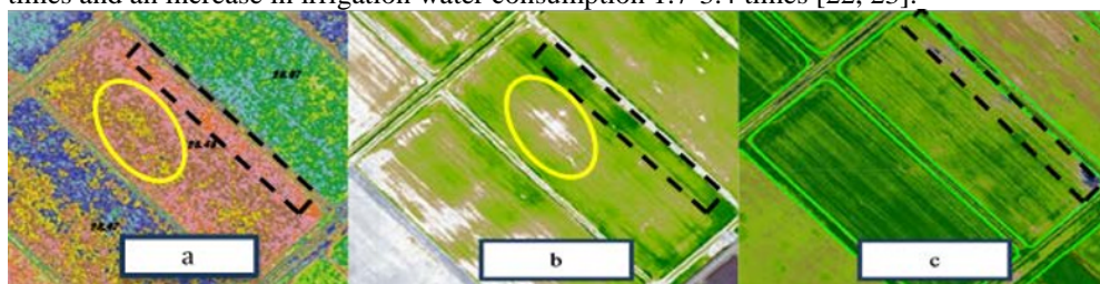
Fig. 6. Comparison of the check hypsometry before sowing with the moisture map and NDVI
