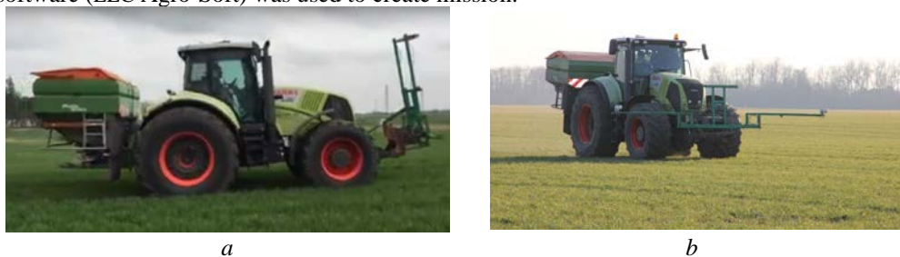
Fig. 2. Differential fertilizer application unit (Claas Axion 850 tractor + Amazone ZA TS 4200 spreader): a-for applying fertilizers using task cards; b - for applying fertilizers using a nitrogen scanner.
