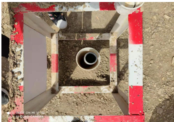
A device for detecting single point settlement on high-speed railway subgrade
