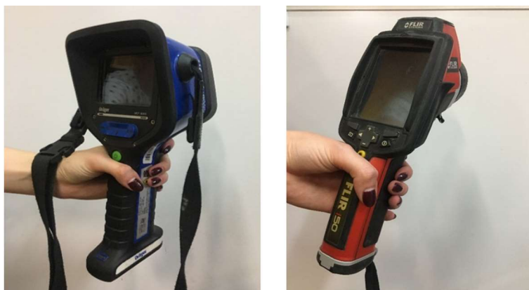
Fig. 2. Thermal cameras used in KWK ROW Ruch Chwałowice.
