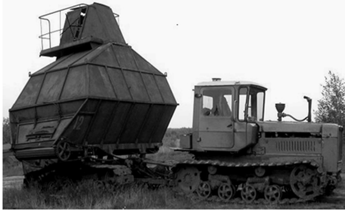
Fig. 2. A scraper-bunker machine with a bucket elevator, equipped with a tracking impeller.
