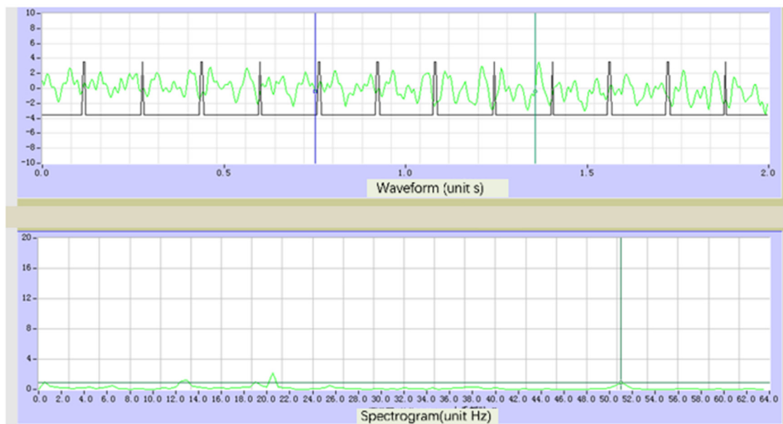
Figure 5. Time-domain waveform and frequency spectrum of axial vibration of thrust support under no-load conditions
