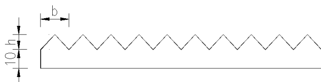
Note: h and b in the figure indicate the height and width of the sawtooth, respectively
