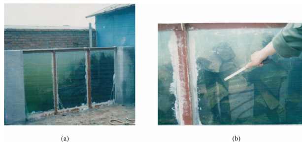
Fig. 8. Model box used in the laboratory tests, (a) model box and (b) conditions of the rockfill.
