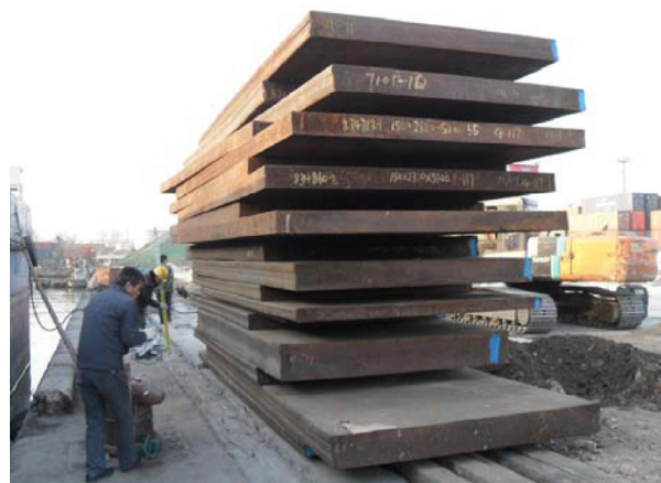
Fig. 17. Pile load test in the gravity wharf in 2010.
