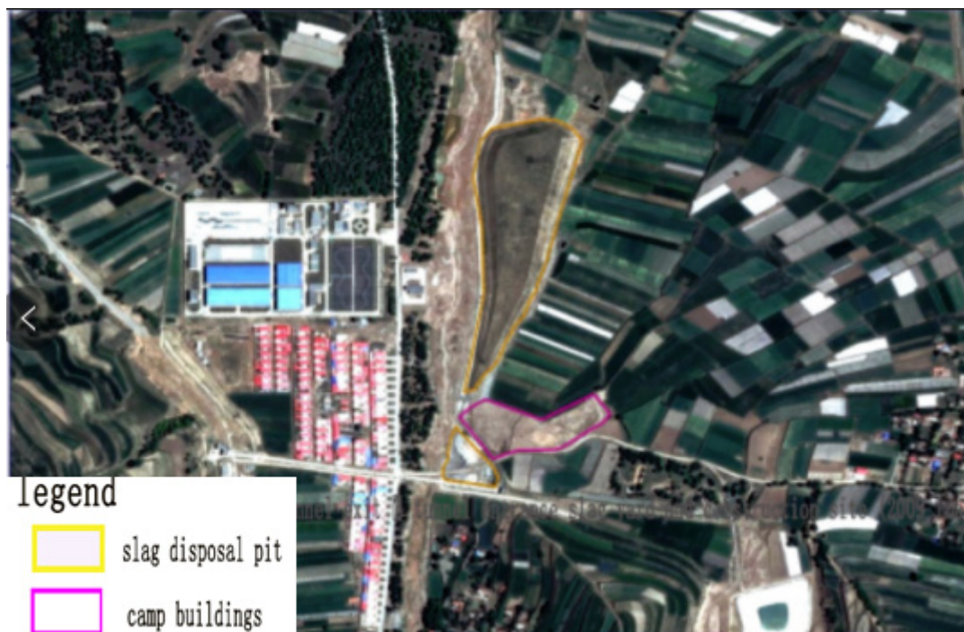
Slag dump and construction site at 10# tunnel entrance of main canal (image in 2018)
