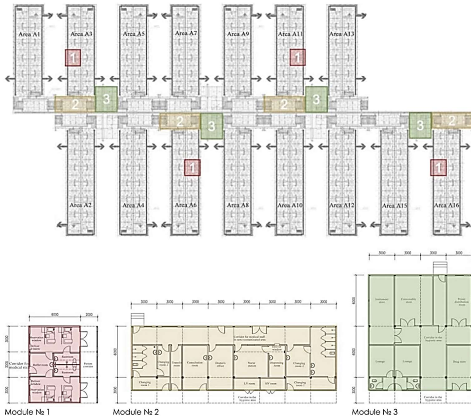
Fig. 4. Functional subdivision of modules [7].
