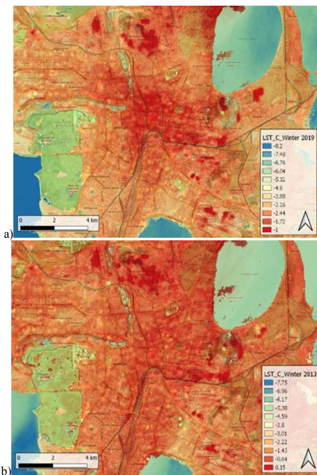
Fig. 8. Image of Chelyabinsk in the thermal range (Band10) of the Landsat 8 system with composite overlay in different mixing modes a) for December 2013 and b) for December 2019.
