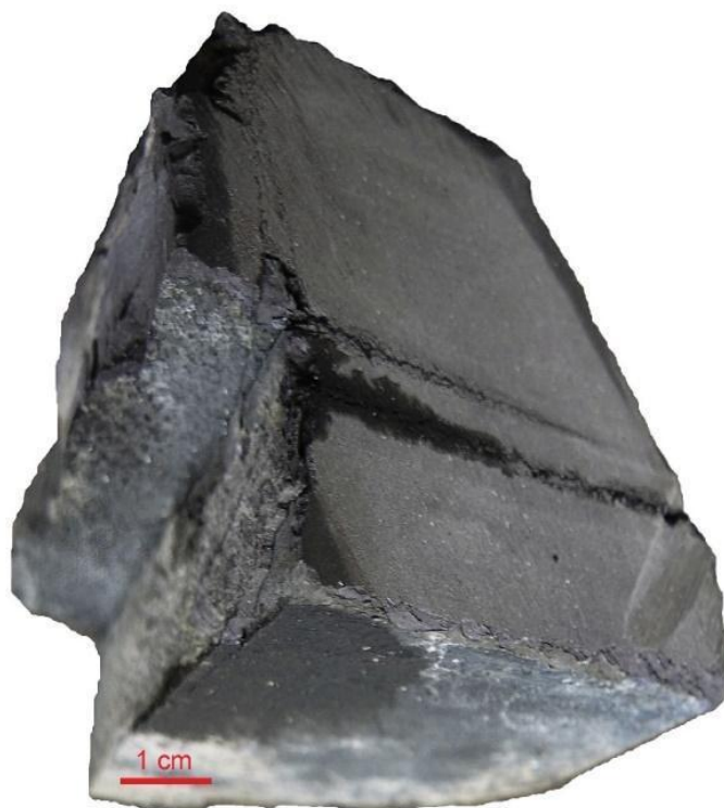
Fig. 7. Hydrocarbon effusion along the fracture.
