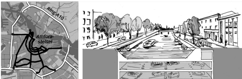
Fig. 6. Diagram of the Amfora Project (left). The layout of the parking space under the canal in the Amphora Project(Internet source 2019).
