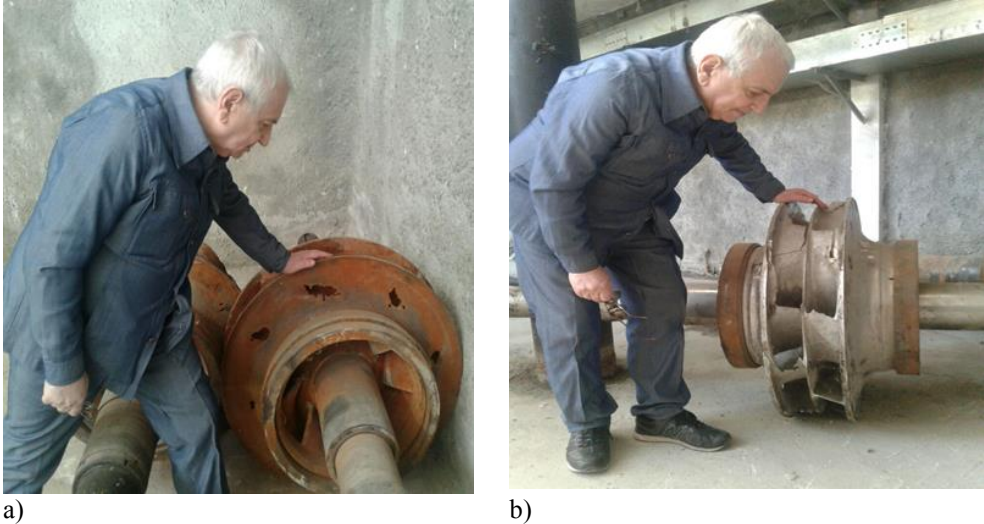
Fig. 2. Analysis of cavitation wear of the pump SPNP80-700SI CD
