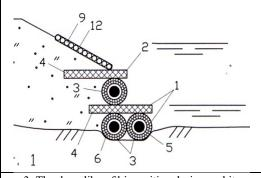
The supporting wall is two-stage and is made of 3 heavy fascines and 4 gabion mats. On the slope above the wall, an attachment is arranged from 12 mats made of 9 wiepped fascines. It is recommended for use against collapse and for restoration of coastal slopes under conditions:
