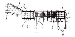
Wooden spatial crib structure 1 is filled with gabion mats 2. The head of dam dikes is reinforced with wooden piles 6. The structure is anchored 8. It is recommended for channel regulation and coastline stabilization under conditions:
