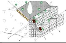
A two-stage supporting wall made of gabions 3, reinforced with reinforcing cage 1. Gabions have 5 stone filling and 6 inclusions from bags with plant soil. It is recommended to use it against erosion and collapse of slopes under conditions:
