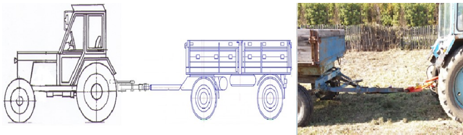
Fig. 2. Connection diagram of a trailer with a tractor through a hydraulic adjustable towing device
