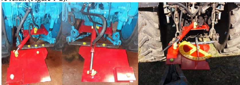
Fig. 1. Experimental hydraulically adjustable towing device
