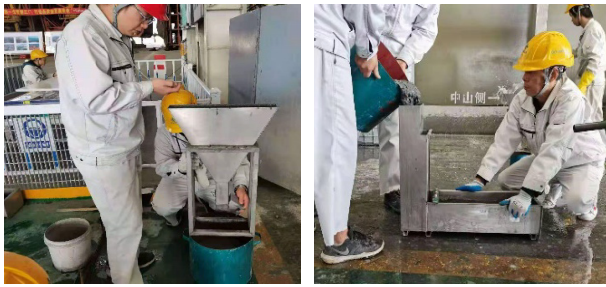
(c) V-funnel test (d) L-box test Fig.1 Working performance measurements for SCC
