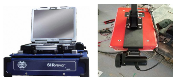
Fig.2 Ground penetrating radar image
