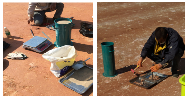
Fig.1 Subgrade compaction detection on site
