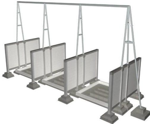
Fig. 7. 3D digital model of Prefabricated Firewall
