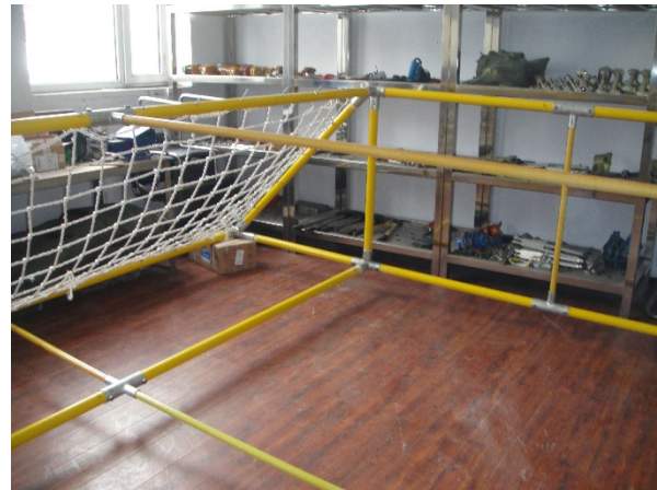
Fig. 3. Insulation protection frame physical assembly picture
