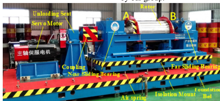
Figure 1. Large-scale rotor test-bed
