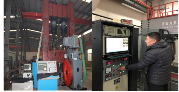
Figure. 3 Zero drift calibration test diagram
