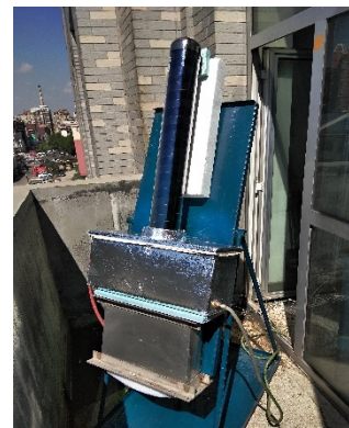
Fig.4 The Bottom-Cooling PHP in Solar Collector
