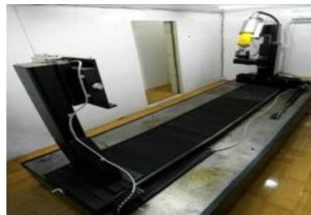
Fig.1. The micro-CT system
