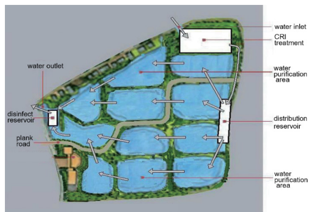
Fig. 2. Plan of sewage treatment system.
