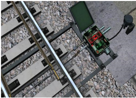
Fig. 4. Result of Unity3D engine rendering ZD6 DC electric switch machine(exclusion state)
