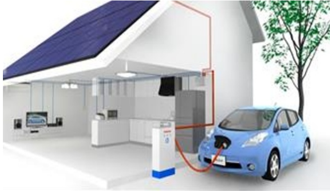
Figure 10: Charging an electric vehicle in a DC home
