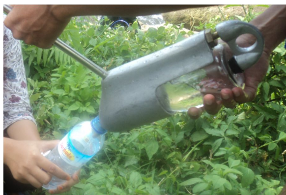
Fig. 6. Removal of sediment from US DH 48
