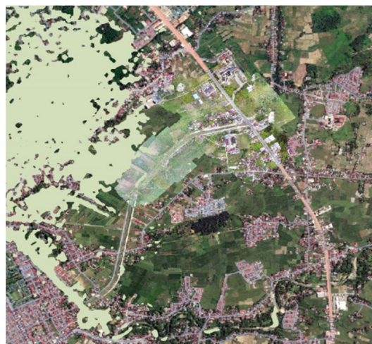
Fig. 9. Flood modeling results of conditions after river normalization with 50 years period in Batang Maransi River.
