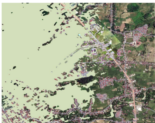
Fig. 7. Flood modeling results of conditions before river normalization with 100 years period in Batang Maransi River.
