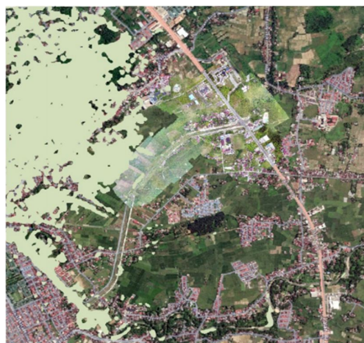
Fig. 10. Flood modelling results of conditions after river normalization with a 100 years period in Batang Maransi in Batang Maransi River.
