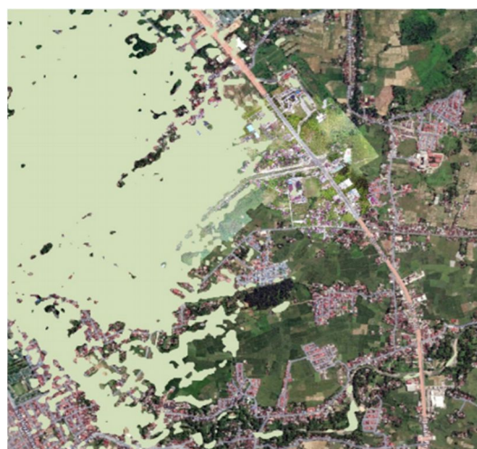
Fig. 5. Flood modeling results of conditions before river normalization with 25 years period in Batang Maransi River.
