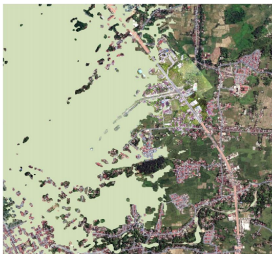
Fig. 6. Flood modeling results of conditions before river normalization with 50 years period in Batang Maransi River.
