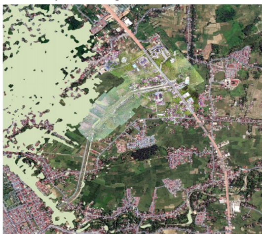
Fig. 8. Flood modeling results of conditions after river normalization with 25 years period in Batang Maransi River.
