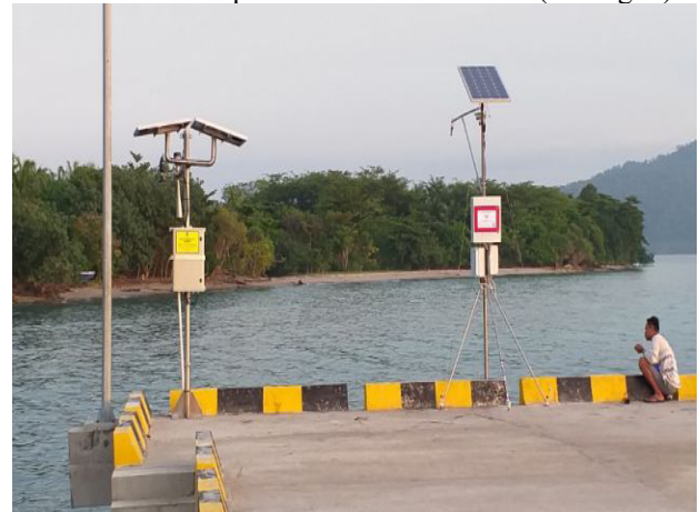
Fig. 3. On the left is the BIG Tide Gauge installation and on the right is IDSL. Both are in Sebesi Harbor.
