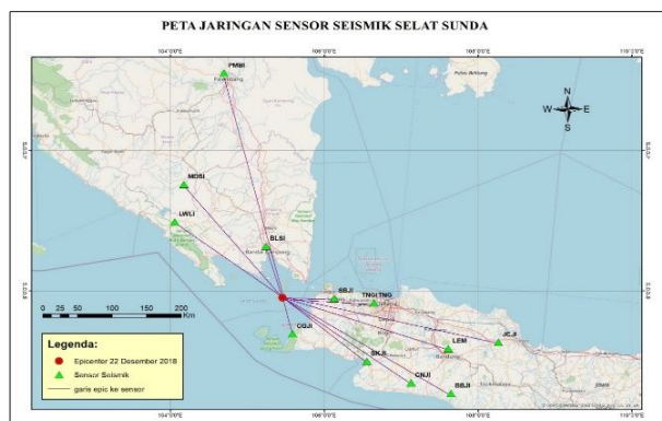
Fig. 12. Center for non-tectonic seismic vibrations from BMKG seismic network monitoring
