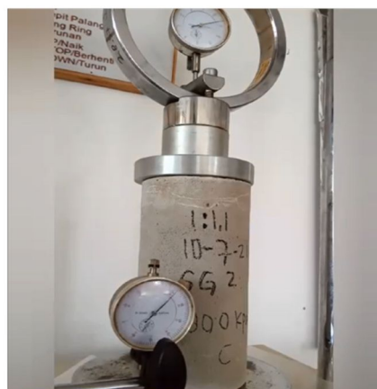
Fig. 4. Modified CBR Equipment
