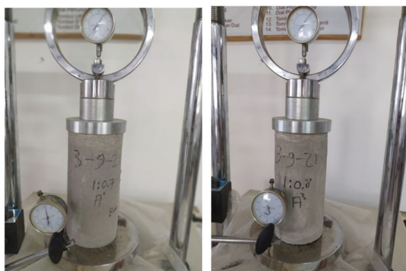
Fig. 5. Compressive test of sample 1C:0.7S & 1C:0.8S
