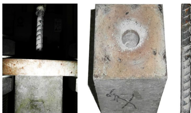
Fig 1. Bond Failure Pattern of Specimen Observed Experimentally [1]
