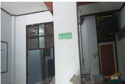
Fig. 8. Example of a misused symbol on Building A, here the same symbol as evacuation one was used to give information of direction to a study program, which on a panic situation it might be misinterpreted as an evacuation route.
