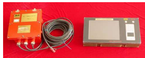
Fig.6 Wireless measuring system (outside hole part)
