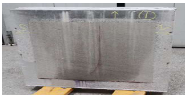
Figure 2. Fracture morphology without natural fractures
