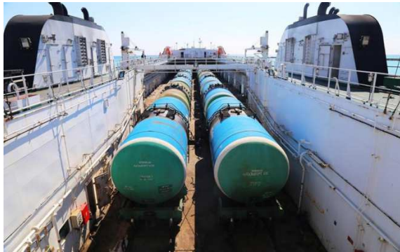
Figure 9. Transportation of rail tank cars by ferryboat
